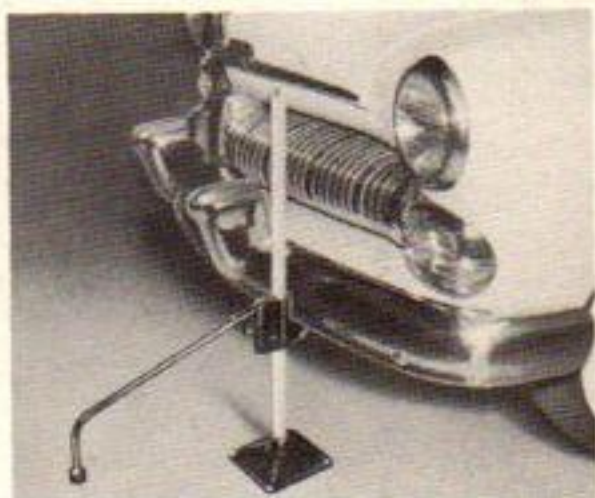
Put V-notch under edge of bumper
