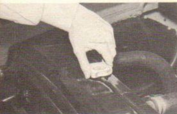
Turn radiator cap to "partly open" stop
