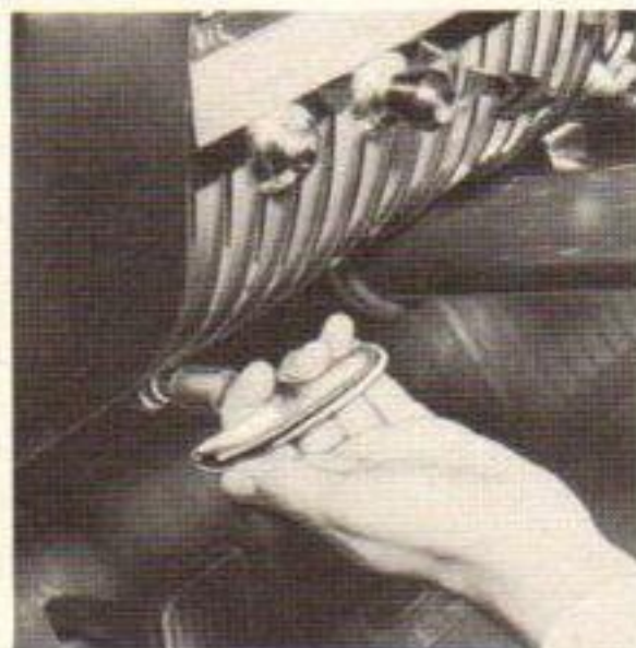
Pull out parking brake to set brakes
