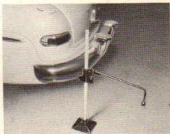
Put V-notch under edge of bumper
