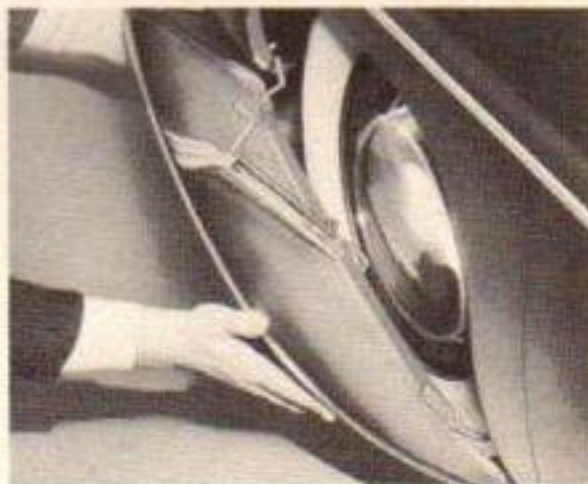
Push wheel cover in to free "guide" rod
