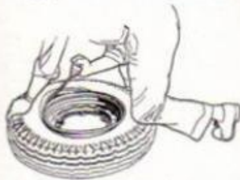
Fig. 28—Applying Top Bead
