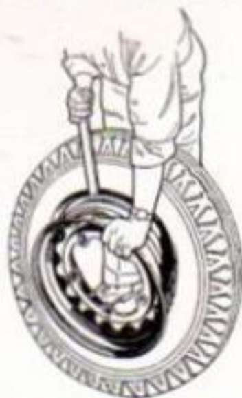
Fig. 26—Removing Bottom Bead
