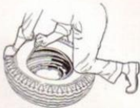
Fig. 27—Applying Bottom Bead
