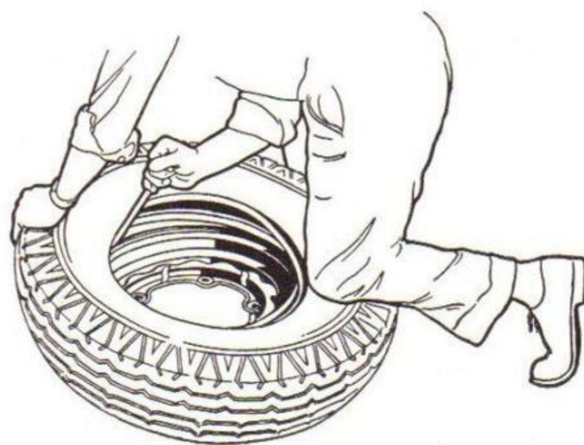
Fig. 27—Applying Bottom Bead
