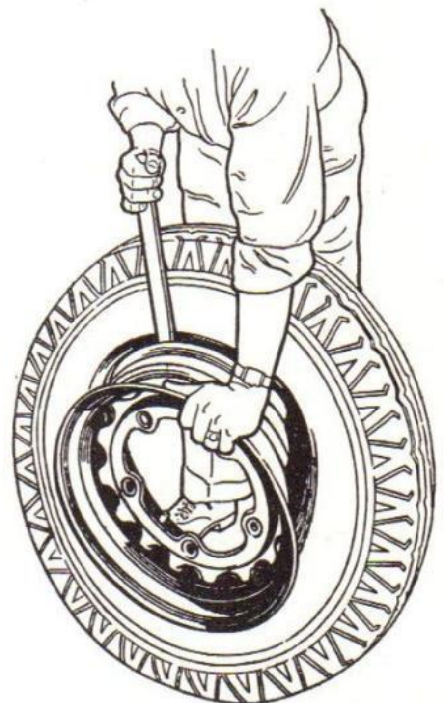
Fig. 26—Removing Bottom Bead
