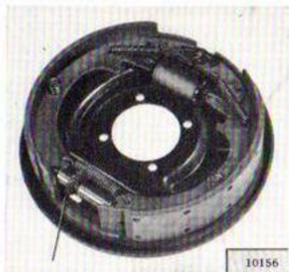
FIG. 29—BRAKE ADJUSTMENT DUAL-REAR-WHEEL MODELS
