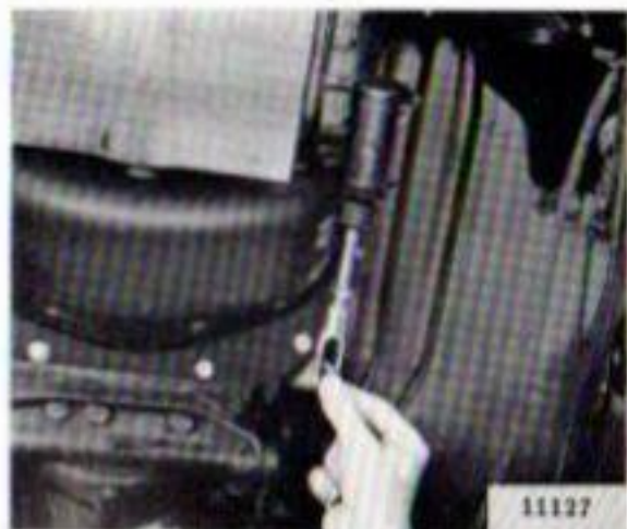
FIG. 25—CLUTCH FREE PLAY ADJUSTMENT
