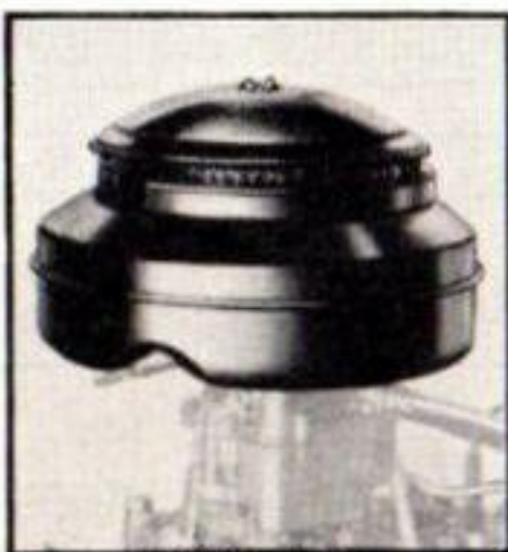
2000 MILES AIR CLEANER—STANDARD Wash In Gasoline And Lubricate With Engine Oil AIR CLEANER—OIL BATH Remove And Wash In Gasoline Pour 1 Pint Engine Oil In Cleaner Body
