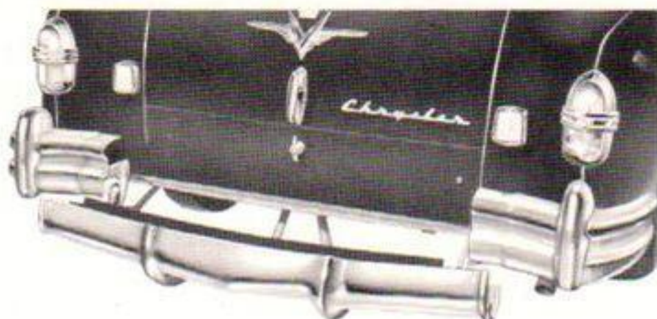
CENTER BUMPER SECTION IN LOWERED POSITION (CROWN IMPERIAL LIMOUSINE)
