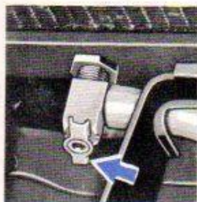
RADIATOR DRAIN COCK
