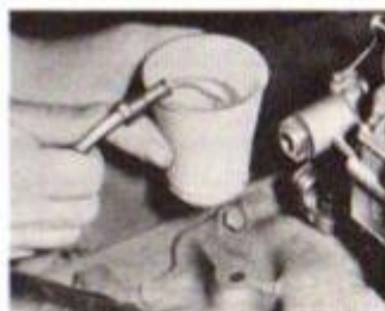
Checking Fuel Flow
