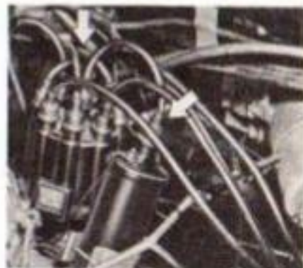
Distributor and Coil Cables
