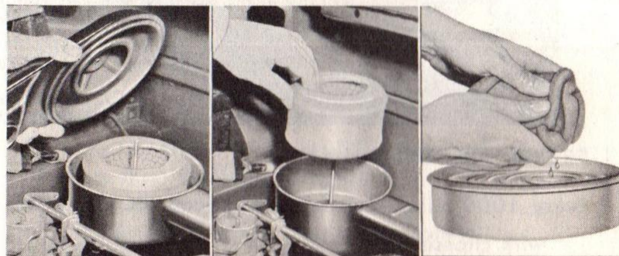
REMOVAL AND CLEANING OF ELEMENT
