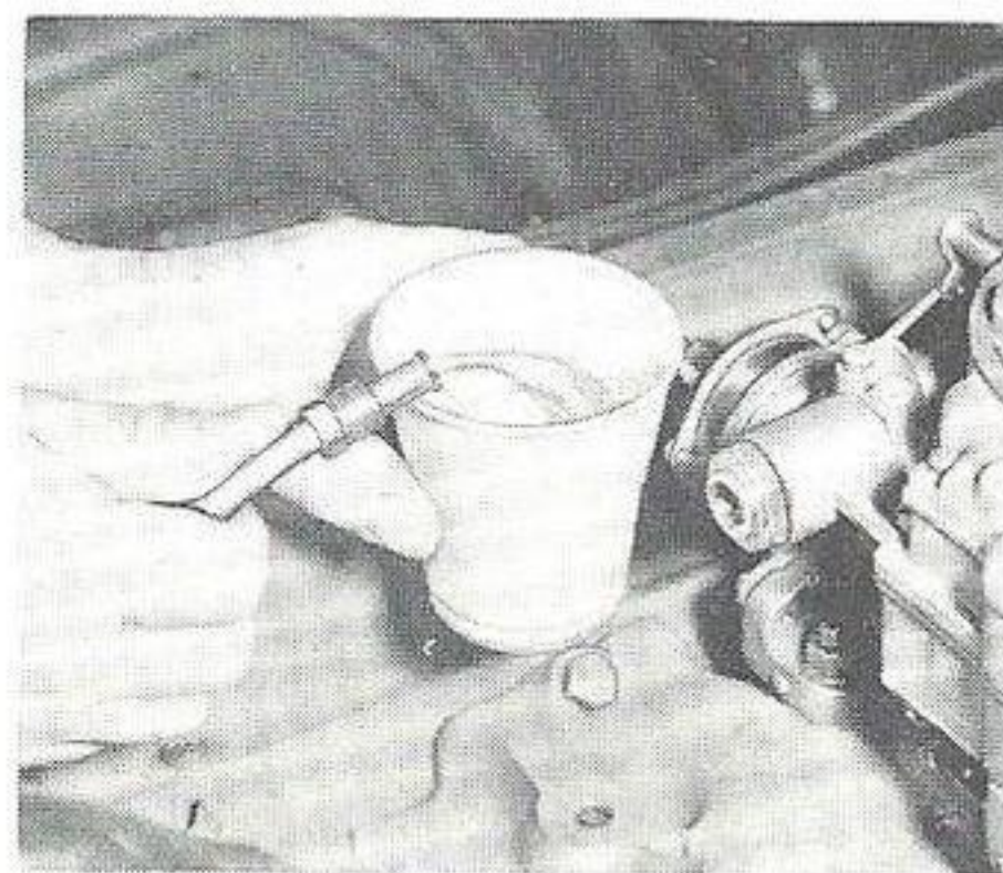
Checking Fuel Flow
