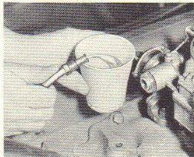
Checking Fuel Flow
