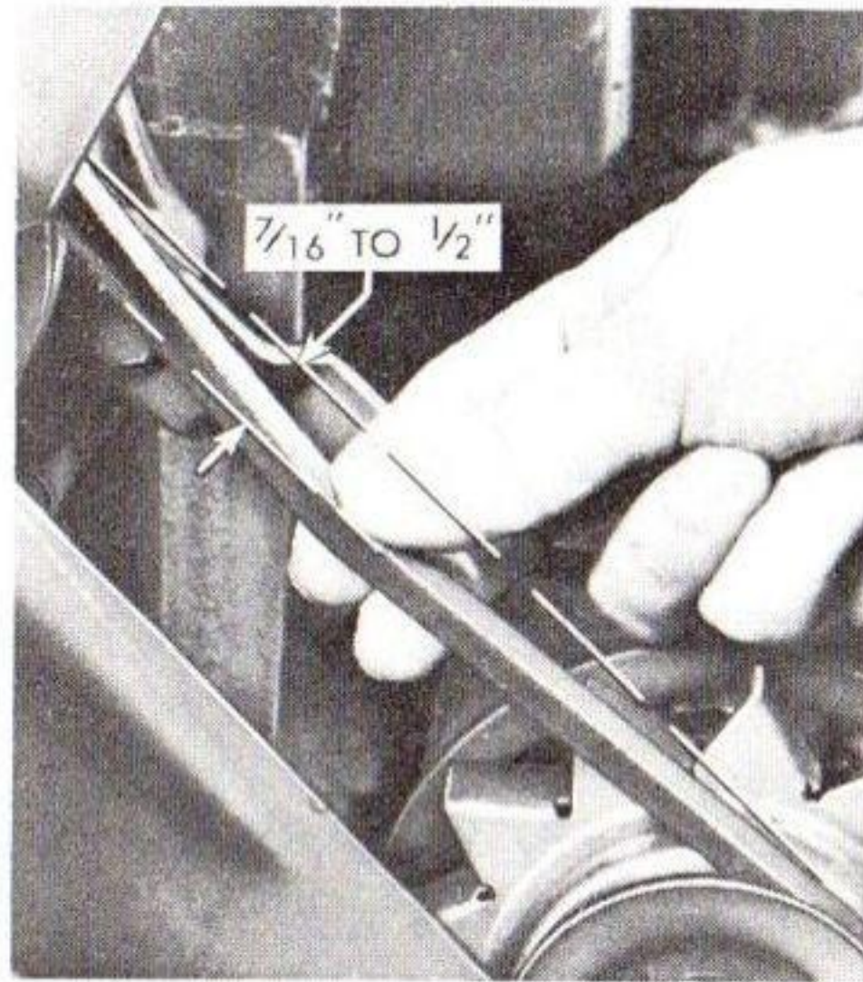
Fig. 71—Fan Belt Adjustment
