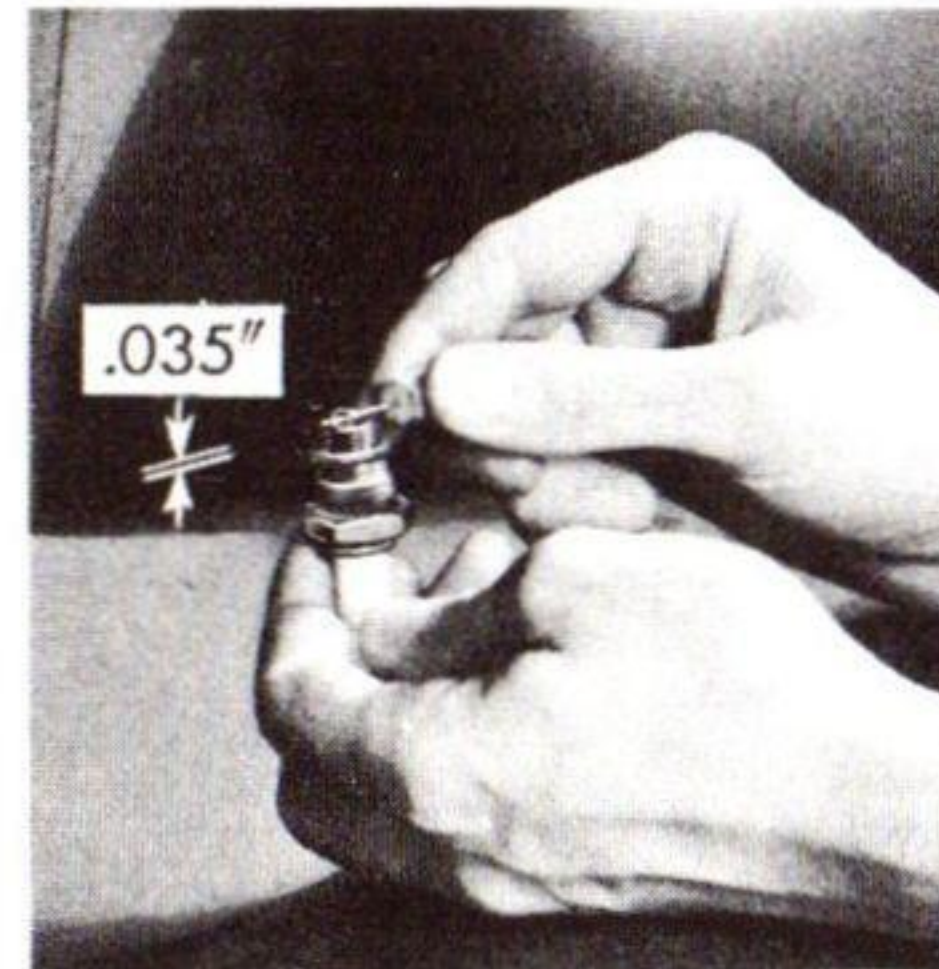
Fig. 63—Setting Spark Plug Gap
