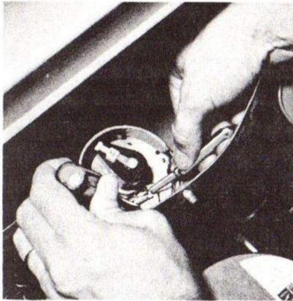
Fig. 66—Adjusting Distributor Points
