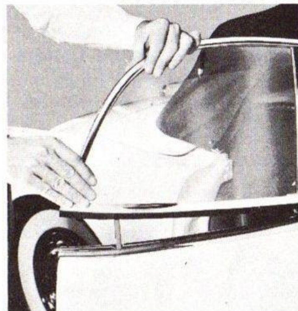
Fig. 35—Lowering Rear Extension
