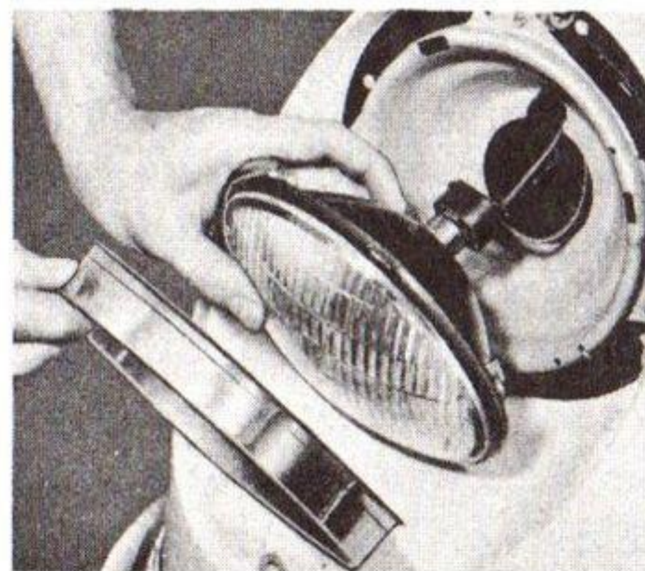
Fig. 77—Removing Retaining Ring and Sealed Beam Unit
