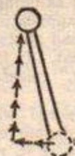
Fig. 11—Sketch showing gear shifting lever being moved from neutral to reverse.
