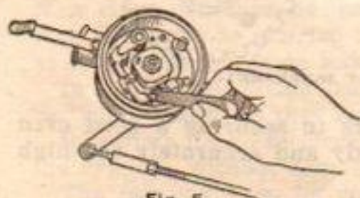
Fig. E. Close contacts and square points by moving file up and down three or four times
