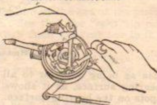
Fig. F. Adjusting contact points
