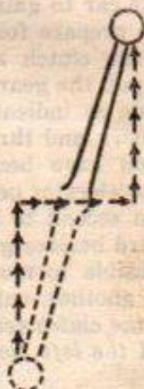
Fig. 9— Sketch showing gear shifting lever being changed from low to second speed.
